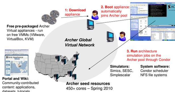
Figure 1. Using Archer for computer architecture simulations. Users can download the Archer VM and boot it using a virtualization software like VMware player or Virtual Box. Within minutes of booting up, the VM automatically joins the existing Archer pool. Users can then submit their jobs from their Archer VM to the nodes in the Archer pool.
