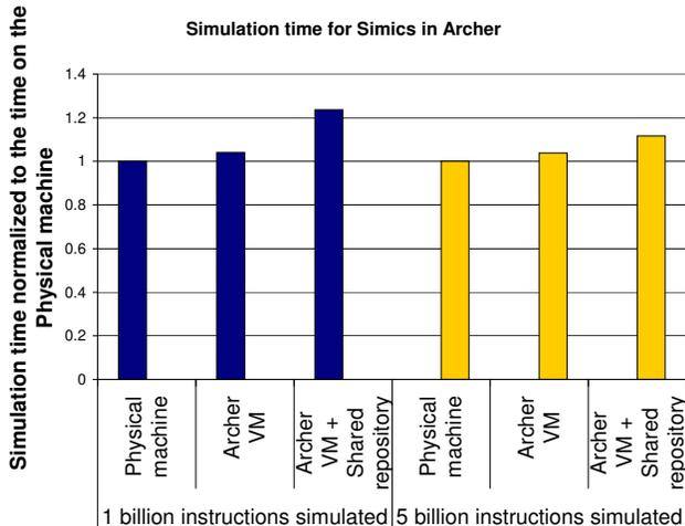
Figure 2. The simulation speed of Simics, with the checkpoint present on the same VM, reduces on on Archer VMs by less than 5%. Even when checkpoints from shared repositories are used over a 100Mbps link, the slowdown is about 11%. This slowdown is smaller for simulations which are less I/O-intensive.
