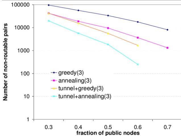
**Fig. 11** Average number of non-routable pairs in a scenario where 20% of NATed nodes are behind symmetric NATs. When 70% of nodes are behind NATs, the percentage of non-routable pairs for greedy and annealing routing is (1) without tunnel edges, 5.6% and 1.88% respectively; (2) with tunnel edges, 1.6% and 0.57% respectively. When 70% of nodes are public, there are no non-routable pairs with tunnel edges
