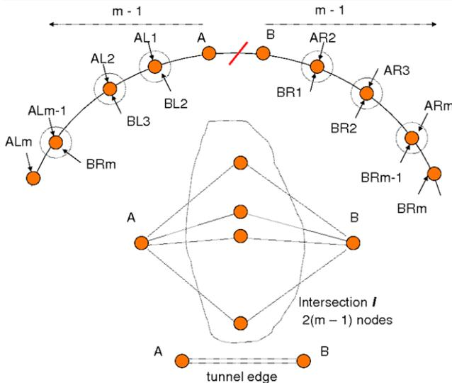
**Fig. 5** Tunnel edge between nodes A and B that cannot communicate over TCP or UDP transports
