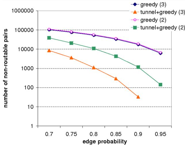
**Fig. 8** Comparing greedy routing with tunnel edges for  $m = 3$  and  $m = 2$ . At edge likelihood of 70%, the percentage of non-routable pairs in a network of 1000 nodes is (1) 3.9% for  $m = 2$ , and (2) 0.86% for  $m = 3$
