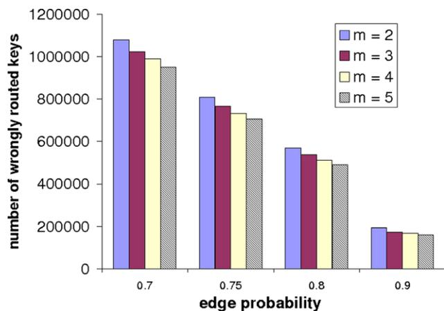
**Fig. 7** At edge likelihood of 70%, the percentage of wrongly routed keys varies from 9.5% to 10.7% (the total number of simulated messages is 10,000,000)
