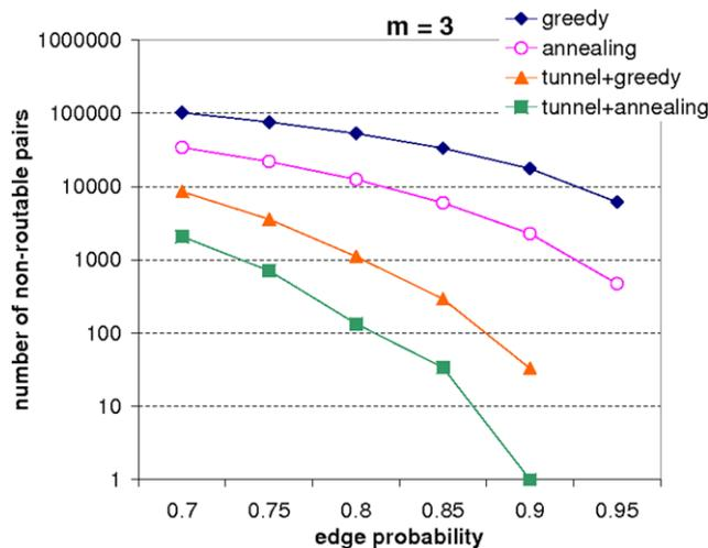
**Fig. 9** Average number of non-routable pairs. At edge likelihood of 70%, the percentage of non-routable pairs for greedy and annealing routing is (1) without tunnel edges, 10.26% and 3.4% respectively; (2) with tunnel edges, 0.86% and 0.21% respectively. At edge likelihoods of 95%, there are no non-routable pairs with tunnel edges
