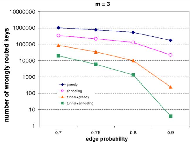
**Fig. 10** Average number of wrongly routed keys. At edge likelihood of 70%, the percentage of wrongly routed keys for greedy and annealing routing is (1) without tunnel edges, 10.2% and 3.4% respectively; (2) with tunnel edges, 0.86% and 0.19% respectively
