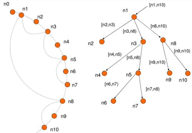
**Fig. 12** Illustration of the use of bounded broadcast over a segment of the P2P ring to search for public nodes. *Left*: a segment of the P2P ring. *Right*: the resulting tree for a bounded broadcast on  $[n1, n10]$
